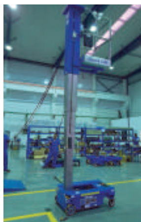
150% Load With 2 Degree Tilt Test
