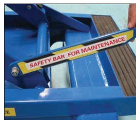
Maintenance safety bars
